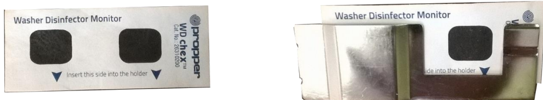
FIGURE 1. PROPPER WD-CHEX INDICATORS. LEFT IMAGE SHOWS LOOSE INDICATOR STRIP. RIGHT IMAGE SHOWS STRIP IN DESIGNATED HOLDER.
