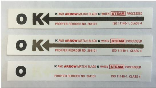
Typical “Pass”(Top), “Fail (Middle), and unprocessed OK<sup>®</sup> and Short OK<sup>®</sup> indicator strips (Bottom).
