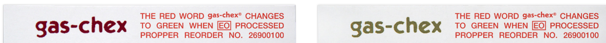
FIGURE 2. LEFT IMAGE SHOWS UNPROCESSED LOOSE INDICATOR STRIP. RIGHT IMAGE SHOWS PROCESSED LOOSE INDICATOR STRIP.
